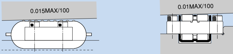
Ⓐ Parallelism between the LM Roller and the raceway Ⓑ Allowable tilt of the roller in the longitudinal direction
