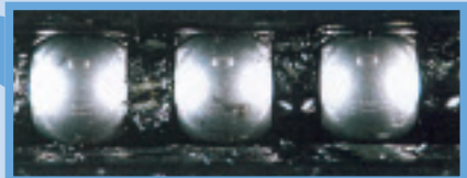
Detail view of the ball cage
