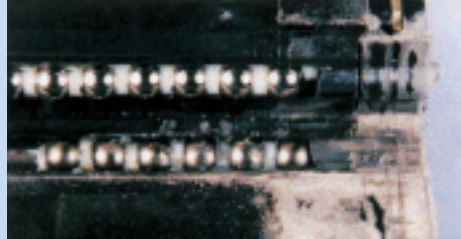
Large amount of foreign matter has entered the ball raceway
