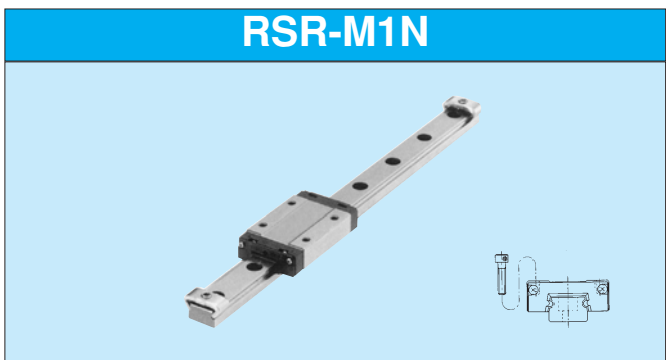
Compared to type RSR-M1V, this type has larger load rating provided by the longer overall length of LM block and increased number of effective balls.
