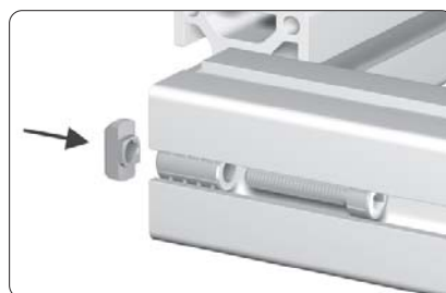
pre-mounting of the T-slot nut
