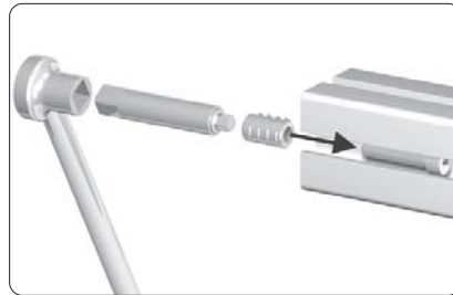
insert the cap head screw and the notching case into the slot
