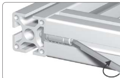
join the profiles and tighten the T-slot nut
