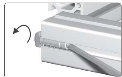
pre-mounting of the T-slot nut
