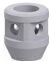
Threaded connection To be screwed to gripping tool Max 160 Kg (D23000304036)
