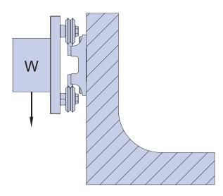
Figure 9: Linear guide configured primarily radial load.
