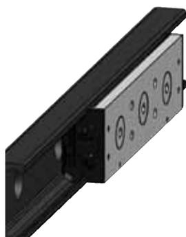
**RLS Series Sliders** The RLS Series Sliders have a very slim body, as the most compact slider, without sacrificing performance. They also offer both threaded and through hole mounting options (RLS and RLSC). The standard slider body is made from Zinc plated steel but is also available in complete inox. The RLS Series Sliders are available in 2 sizes, 2 materials, and with either 3, 4 or 5 rollers.
