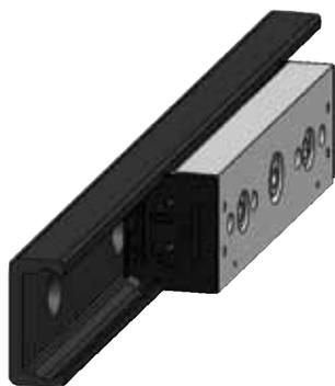
**RLV Series Sliders** RLV Series Sliders are made of strong Zinc plated steel body, with mounting holes parallel to the roller axles and perpendicular to the direction of preferred loading. The sliders have wipers with incorporate preoiled felt for lubrication of raceways. The RLV Series Sliders are available in 2 sizes and with either 3 or 5 rollers.
