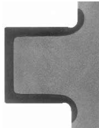
Fig. 15: Raceways of a nose ring in a three-row roller bearing slewing ring.
