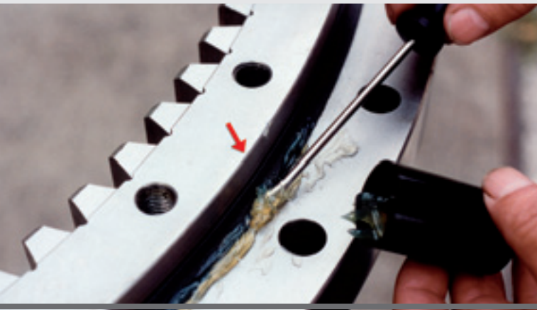
Figure 13: Taking a sample of grease from the sealing lip
