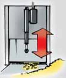
The LA31 actuator is a very quiet and powerful actuator designed for a variety of applications including furniture, care beds etc. It is designed with built-in limit switches.
