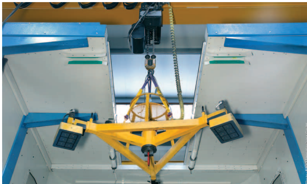
■ Roof opening to supply workpieces by crane.
