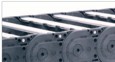
■ Stay variant RMF – stays affixed to each side with 1 screw. Inside/outside: stays can be quickly released for laying cables.
