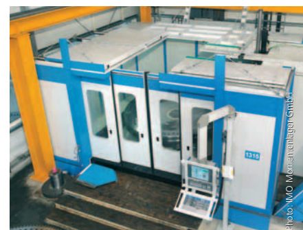
■ Sliding roof elements in different opening positions.
