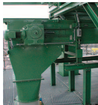
■ Scraper conveyor for distribution of various chip materials
