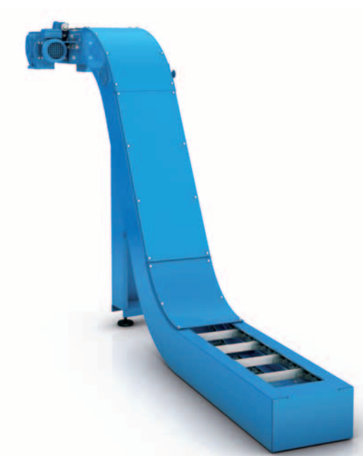
■ Straight/rising/straight design Max. incline 60°
