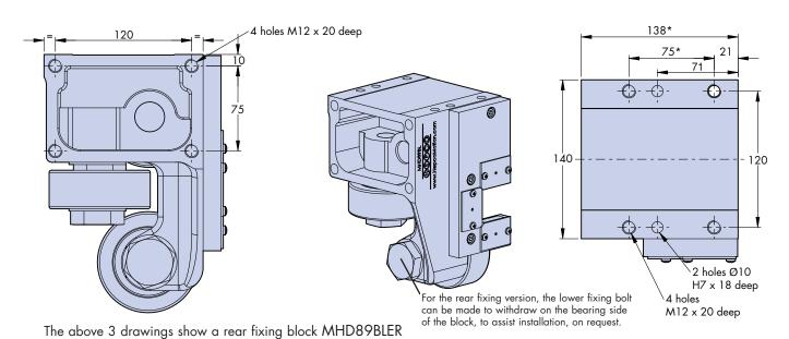
dimensions marked \* differ between the standard and rear fixing variants.
