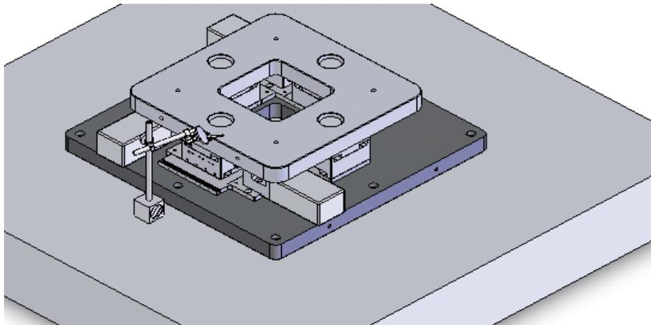
Put the alignment stage onto the bench under inspection; fully make measurements by sliding the test indicator. Now locate the bench at the stroke-middle point. Use the maximum deviation made during the bench-measuring zone as the measuring value.
