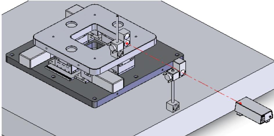
Use the length-measuring laser interferometer to make repetitive positioning procedures for seven times in the same direction at any chosen point and measure the respective stop positions; find half of the maximum deviation. Perform measurements at center and both ends of the moving distance; pick the maximum value as the measured value; and add the "±" to the half of maximum deviation value.
