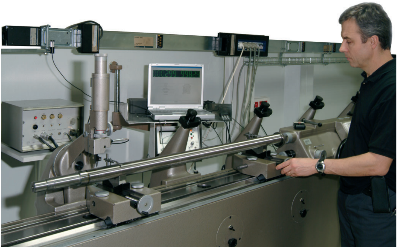
Lead error control interferometric test bench
