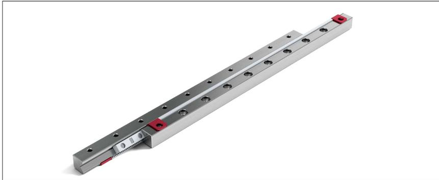
In every linear guideway the cage can be shifted from the centre along the longitudinal axis. Cage creep reduces the optimal load distribution and requires a correct stroke to return the cage to a centered position. The correction stroke requires a large expense of energy.
