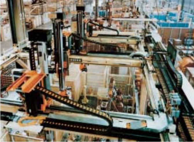
Type 0450 and 0625 Plastic Cable Carriers on an automatic production line at the Friedrichshafen AG Gear Cutting Factory
