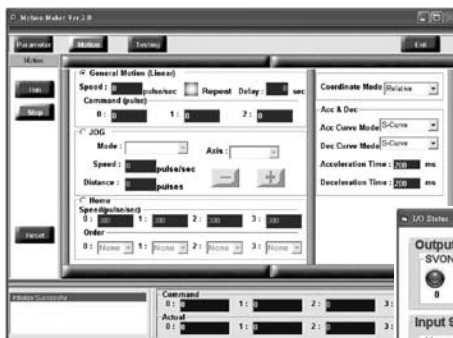
Testing general motions, jog, and homing. Display of I/O status.
