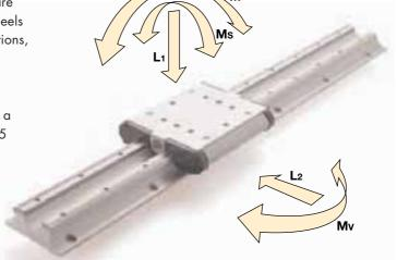
Once the system load has been resolved into the (up to) 5 components of direct and moment load, then the **Load factor** LF can be calculated using the following formula:
